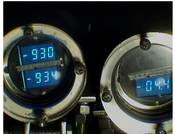
The Deep C Meter in situ mounted to an ROV The ROV II Probe is taking a stab reading
