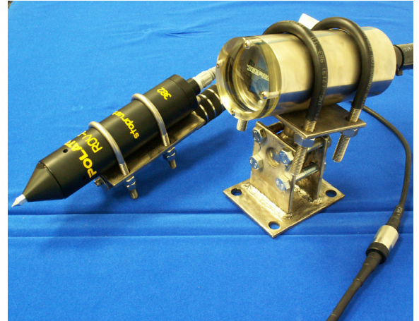
The Deep C Meter Connected to the ROV II CP Probe, mounted on the dynamic ROV mount
